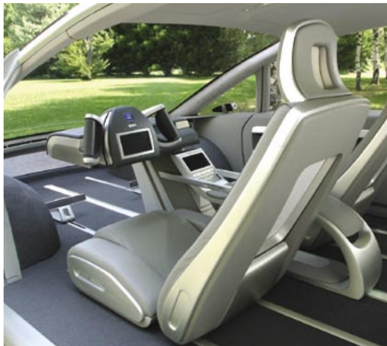
▲ A major advantage of the Hy-wire prototype fuel-cell car from General Motors is that all the propulsion and control systems are in a skateboardlike chassis, maximizing the interior space.
